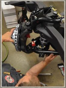
corners. Viking gives guidelines for three different ride types, cruising, handling or drag strip and trust me, this works very well. The Coil-Overs also can be adjusted for ride height. Viking offers these in stock height, lowered or even raised for the gasser look.
