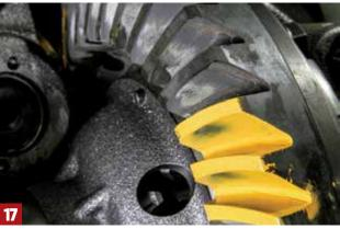
■After a couple of adjustments, the pattern has moved inward on the teeth, indicating this mesh contact pattern is good to go.
