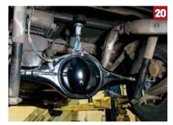
The S-10 is modified with a lift equalizer in the bed, featuring a ring that holds the third member during installation and removal, allowing a pit stop-like changeover from one centersection to the next in about 20 minutes.
