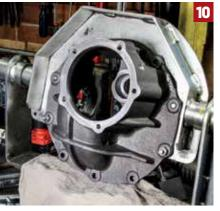
Work moves on to assembly of the third member. starting with a nodular iron case, mounted on a special vise developed by John's Industries. Dubbed the Orbit 480, for its range of motion, it's designed specifically for assembling 9-inch centersections.
