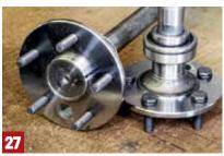
John's machines their own axles, too, from supplied blanks. They prefer screw-in studs versus conventional press-in studs for a few reasons, not the least of which dimensional accuracy and greater safety. They're more secure once they're attached to the axle flange.
