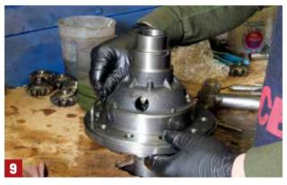
With all of its guts assembled, the Trac-Loc carrier is buttoned up and prepped for installation in the third member.
