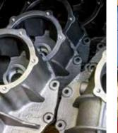
Each third member assembly begins with a nodular iron case or a cast-aluminum case, each available in 3.062-inch and larger 3.25-inch bores. John's Industries' own nodular iron case is made to a unique specification that makes it about 70 percent stronger than factory castings. It's offered with the conventional 3.062-inch bore.
