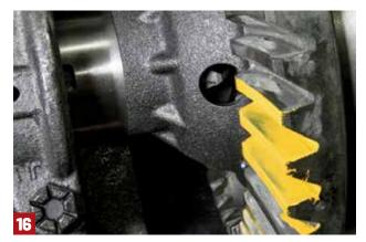
■The first pattern inspection, here, showed the mesh was a little too close to the heel (outer) edge of the teeth. Adjustments are made by adjusting the pinion cartridge shims and re-setting the ring gear backlash. It can take several attempts and shim adjustments to get it just right.
