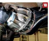
The assembled third member is sent for road testing, where it is installed in the company's test vehicle. The easily removable design of the centersection is one of the things that has always made the 9-inch a favorite with racers and it certainly helps facilitate such tests here.
