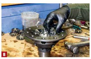
The carrier assembly continues with the installation of the spider gears in the case, which work with the clutch pack in a limited-slip design to reduce the wheel speed of the fastest-turning wheel in order to maintain the same relative speed between the wheels.
