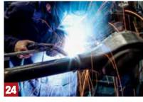
Axletubes are welded to the housing center on a unique, rotating jig that helps produce more consistent welds and does so quite quickly.
