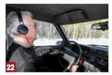
■Inside the test truck, two sets of headphones connected to special sensors mounted in the axlehousing allow technicians to listen to the inside of the axle and note the drive and coast sound levels of the ring-and-pinion. We listened to different assemblies on more than one testdrive and were amazed at the audible variances.
