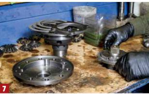
A variety of popular carriers are available, including the company's own Trac-Loc limited-slip unit, which is assembled in-house. It gets started, here, with the carbon clutch pack in the housing.
