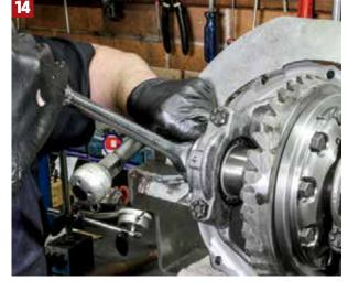
Next, the mesh pattern of the gears is checked, starting with applying some marking compound to a number of the ring gear teeth. Ideally, the pinion should mesh near the center of the face of the rear gear teeth. There's a drive and coast side to the ring gear teeth and the drive side is the more critical side of the mesh pattern.
